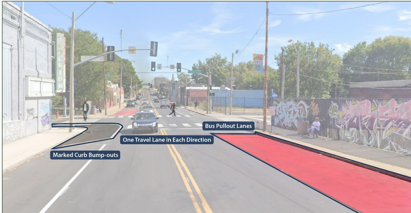
31 st Street Road Diet Source: Google Streetview
