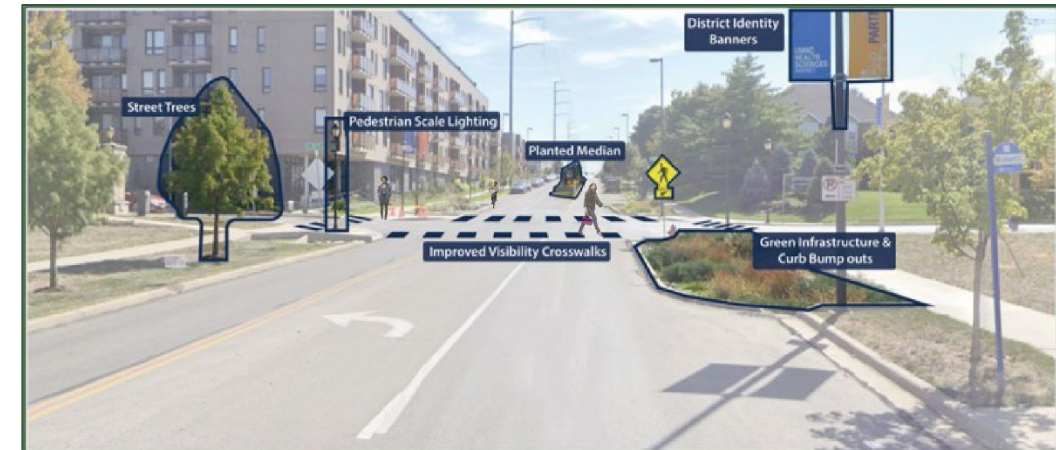
Graphic showing “pedestrian first” infrastructure at 25 th and Troost.
