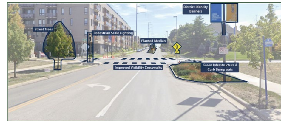
Diagram of Public Space Improvements at 25 th & Troost. Background image from Google Streetview.
